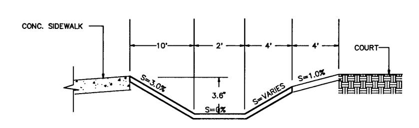
SECTION A-A DRAINAGE SWALE N.T.S.
