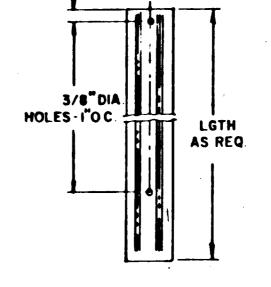
STEEL FOR POST SHALL CONFORM TO MECHANICAL REQUIREMENTS OF ASTM A499 -BI GRADE 60 AND TO CHEMICAL REQUIREMENTS OF ASTM AI - 76 CARBON STEEL TEE RAIL HAVING NORMAL WEIGHT OF 91 LB OR GREATER PER LINEAR YARD.
