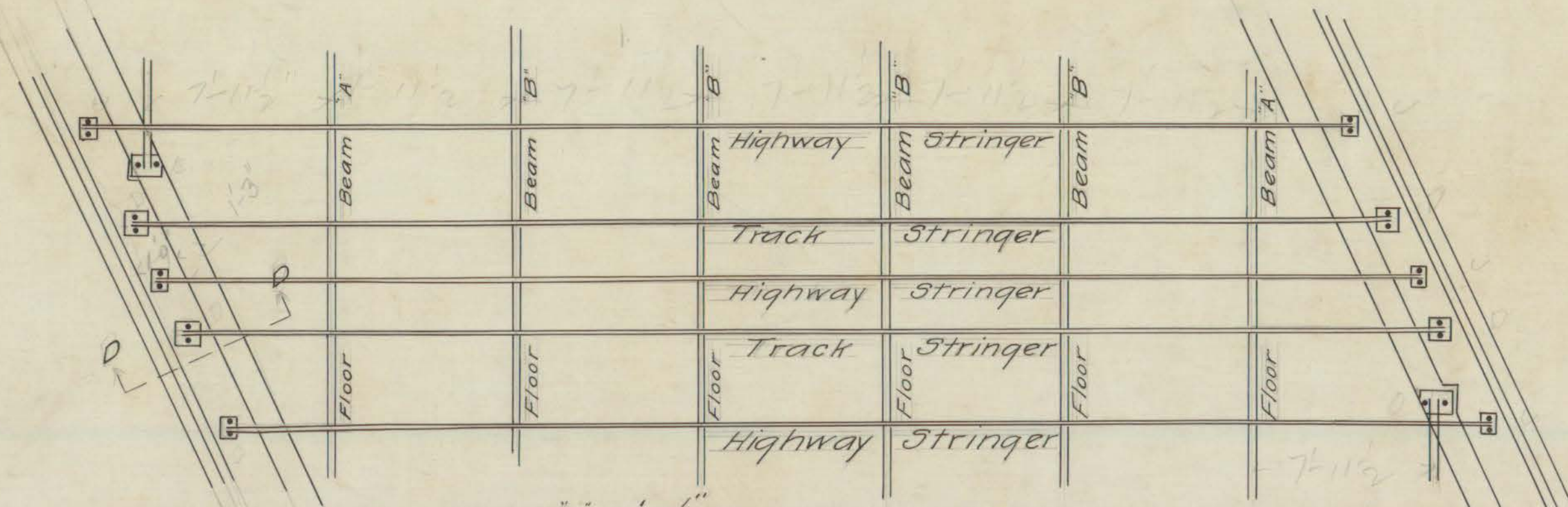
Plan Showing Relative Positions of Stringers and Floor Beams
